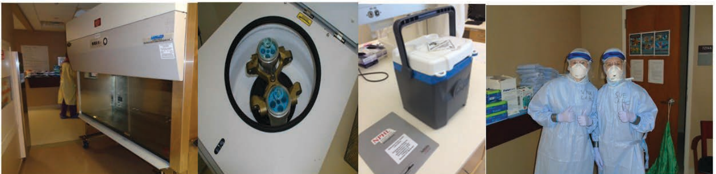
Picture 1. Mobile BSC, Centrifuge with sealed rotors, hard sided transport container, PPE
